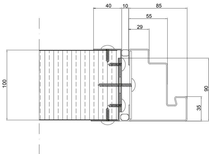
The door was mounted on the support by means of self-tapping screws 5.5x45 mm. Minimum thickness of the support mm 100
