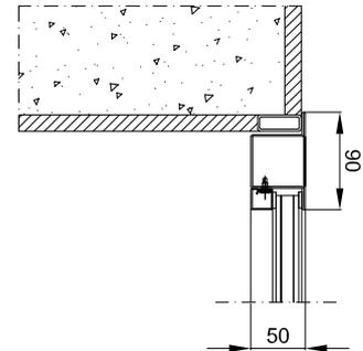
Installation in a T-shaped edge with opposite opening
