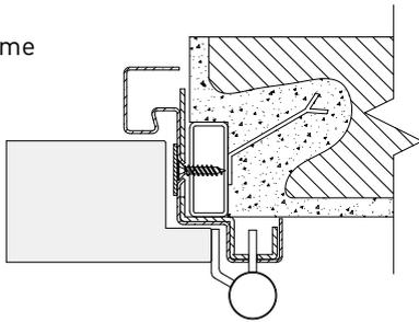
Elite Premio doors are tested on a standardised flexible support, according to the EN 1363-1 standard, par 7.2.2. In accordance with point 13.5.3. of EN 1634-1, the product can be installed in any non-standard flexible supporting construction, which achieves at least the same level of fire performance as the door.
