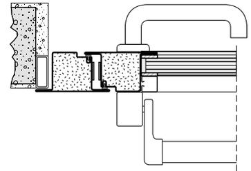
Installation in a T-shaped edge with opposite opening
