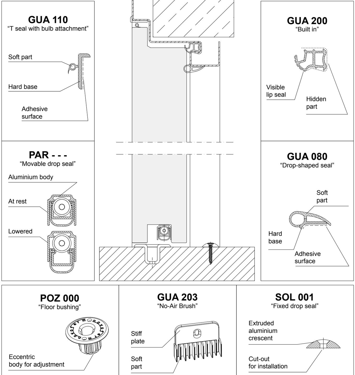
Available fixed thresholds. N.B.: type B and S involve a shortening of the passive leaf rebate.
