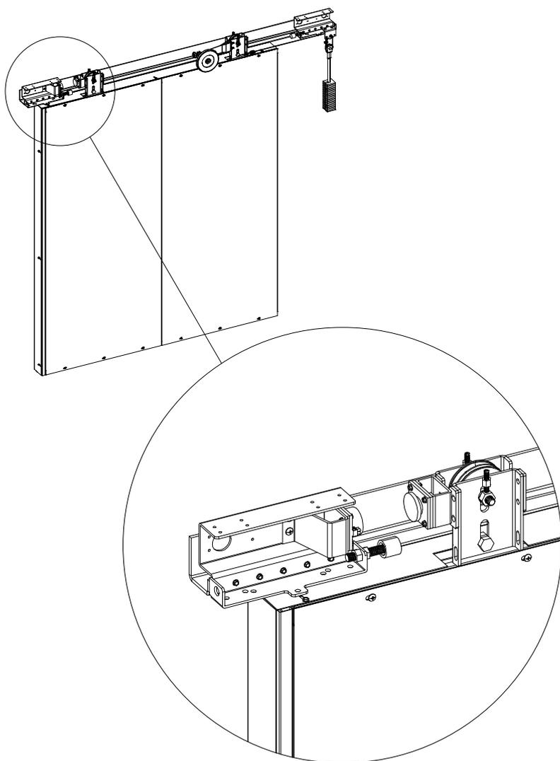
Indicative electromagnet installation diagram
