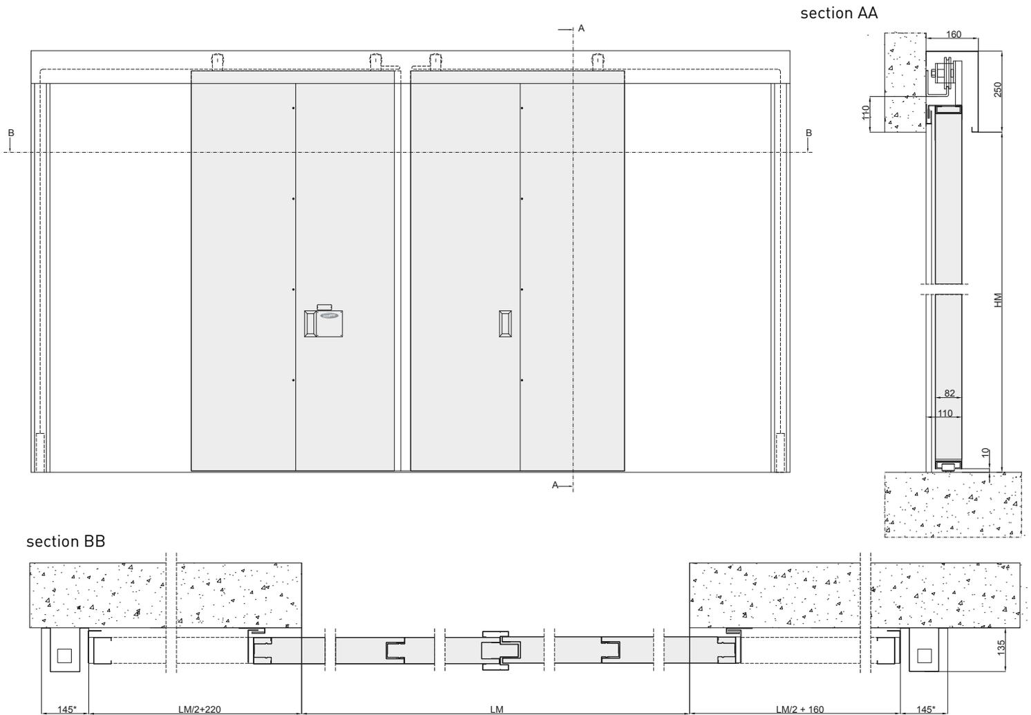
\* Door size with  $HM > LM$ . When  $HM < LM$ , the size of the counterweight can vary from 146 to 290 mm.
