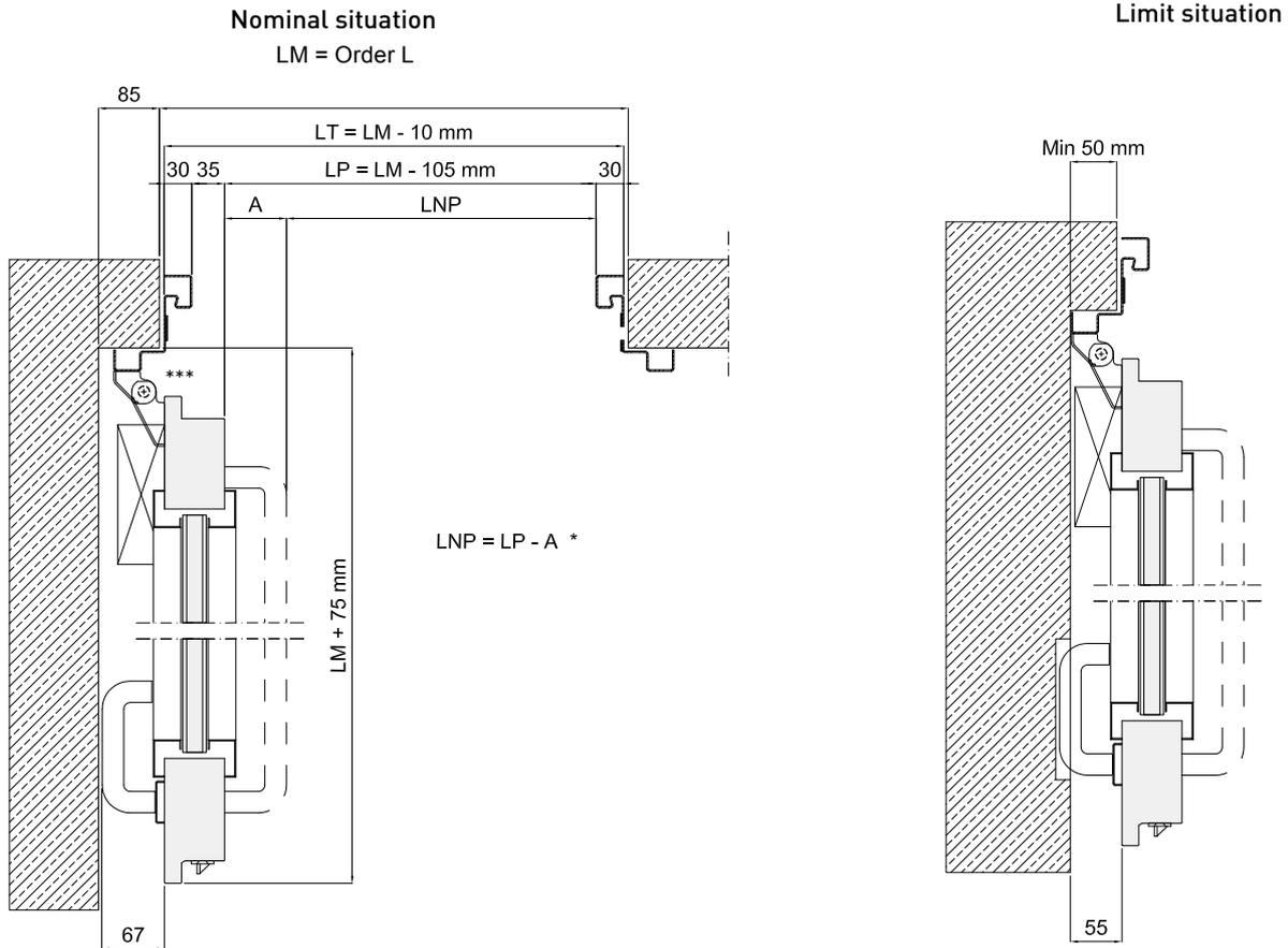
180° opening with steel spring hinge. For standard hinge please see Elite Premio section
