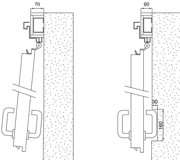
**Installation on insulated flexible panels, tubular frame EI 90,60 and non-fire rated door**
