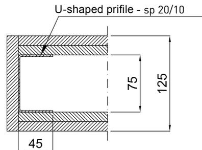
The structure must be covered with gypsum panels with proper quantity and thickness according to construction system adopted.
