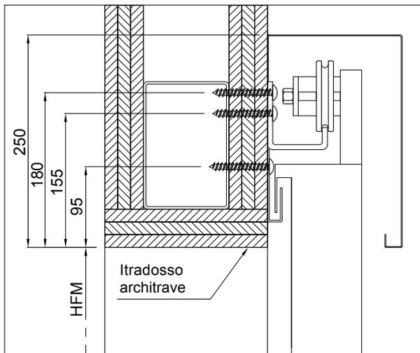
Example of a customer-provided beam coating (not binding). The construction will be projected and realized by the company that performs the compartments (including beam cladding).
