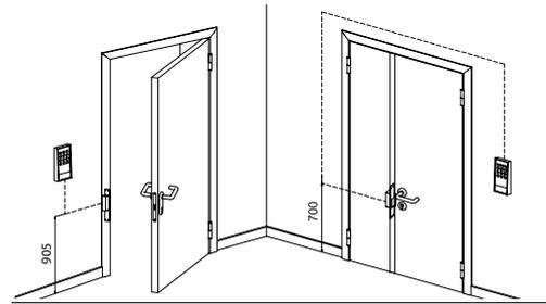
N.B.: The panic bar must be installed on the larger door panel, and not on the smaller one.
