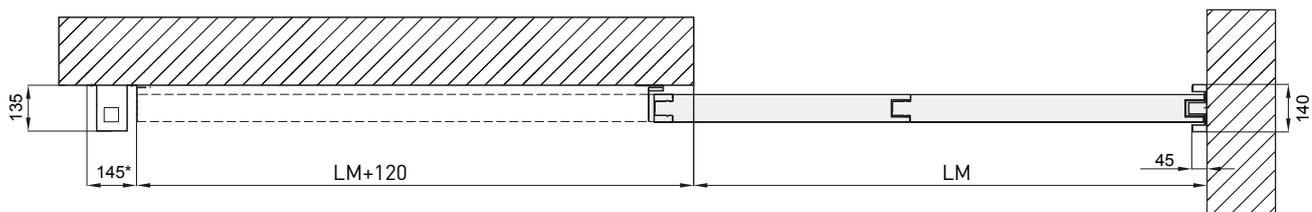
\* Door size with  $HM > LM$ . When  $HM < LM$ , the size of the counterweight can vary from 146 to 290 mm.
