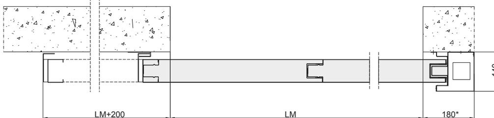
\* Door size with  $HM > LM$ . When  $HM < LM$ , the size of the counterweight can vary from 181 to 340 mm.
